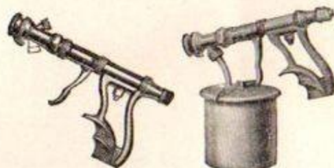
Modern equipment is made for ease of operation and speedy work. Guns have a pistol grip and the paint cups are readily refilled.
